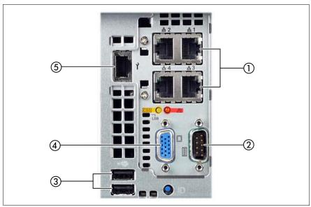
Figure 9: Connectors on the rear
